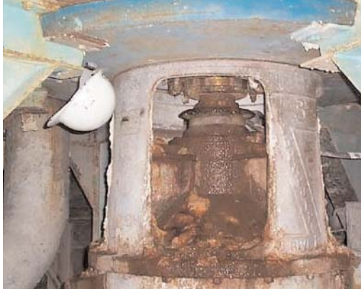
Vertical Shaft of Pulper Unit
