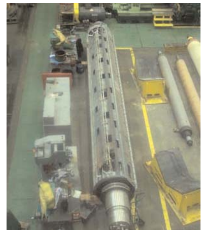
Suction Roller Removed for Maintenance
